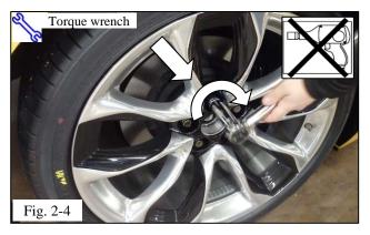
(d) Apply pressure on the key and use a torque wrench to tighten the wheel locks to 140 N·m (103 ft·lbf) (Fig. 2-4).
