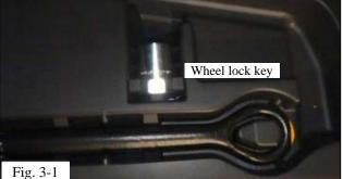
(a) Place the wheel lock key in the foam tool tray (Fig. 3-1).
