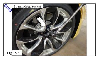
(c) Place the 21mm deep socket on top of the key (Fig. 2-3).
